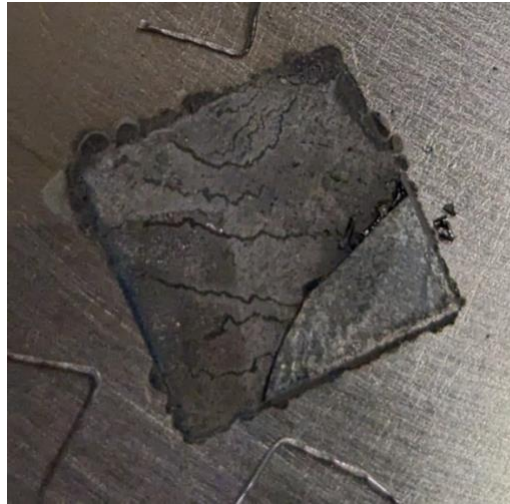
Figure 19. LGS reaction with tantalum holder when heated to 800°C in vacuum showing cracks in the LGS sample.
