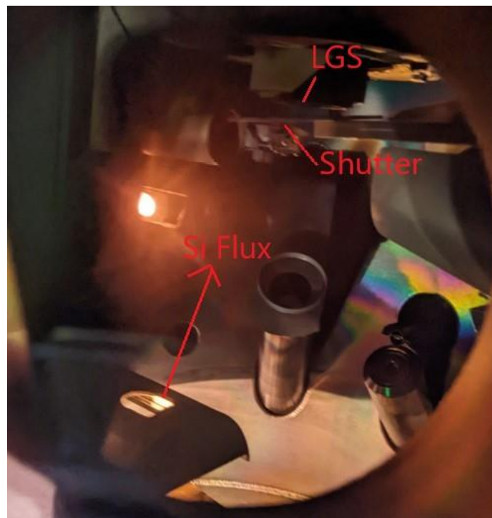
Figure 6. Photograph of EB-PVD system used in experiments.
