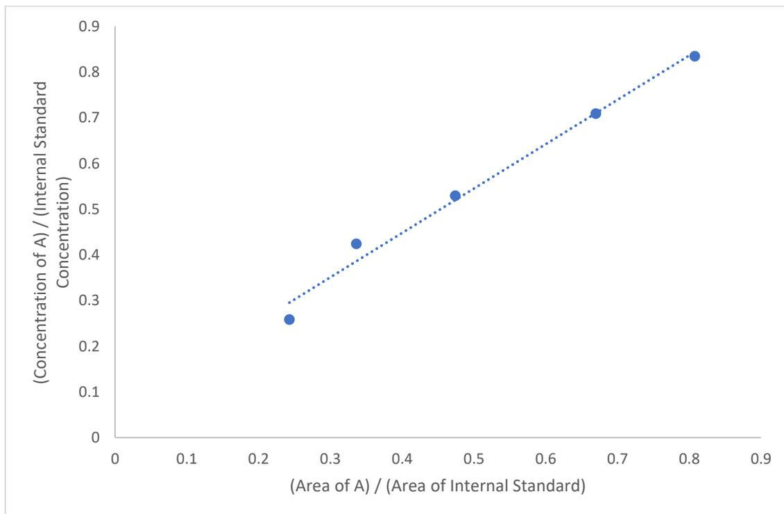
Figure 6. Example of calibration curve used for aqueous reactions. For both concentration and signal area, the ratios of analyte to internal standard are plotted.
