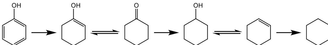
Figure 4. Phenol hydrogenation reaction pathway.
