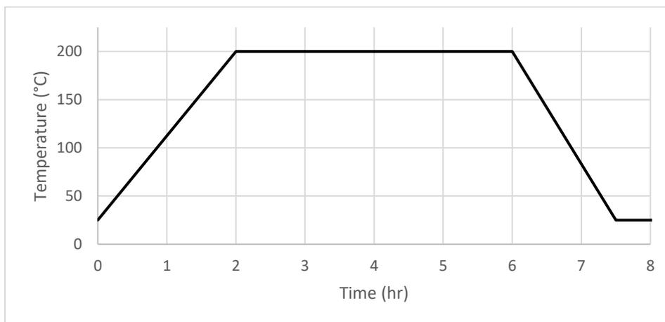
Figure 5. Temperature profile of reaction mixture over reaction time. Time to cool to ambient conditions from hour 6 is approximate.
