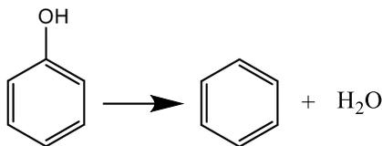
Figure 3. Phenol direct deoxygenation reaction pathway.
