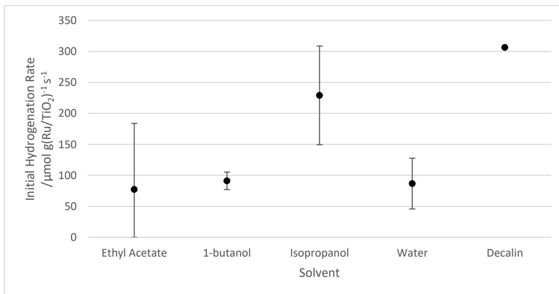
Figure 7. Initial hydrogenation rates in tested solvents. Reactions were performed with initial phenol concentration of 0.53 M in solvent, 33 bar hydrogen pressure, at 200 °C temperature setpoint. Error bars represent 95% confidence interval. Decalin point does not include error bars as only 1 data point was <30% conversion.
