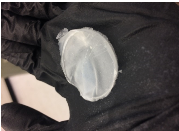
Figure 7 – A CNF film produced via vacuum filtration and removal of water from a raw slurry. The film is stiff and resilient, but the optical transparency is low, and the accumulation of material into spots is notable, especially on the upper portion of the film which is notably lighter.
