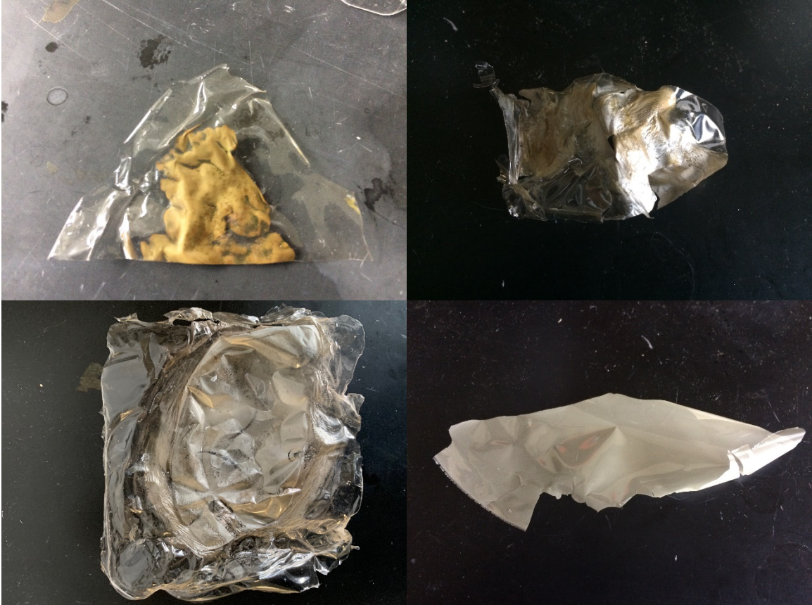
Figure 9 – Clockwise from top-left: TEMPO film treated by the dropping method, with extensive corrosion. A second film treated by dropping, note the wrinkling and light corrosion. A homogenized TEMPO/AgNW film, with no corrosion, even color, and relative lack of wrinkling. Lastly, a film treated with dropping, but corrosion is absent.
