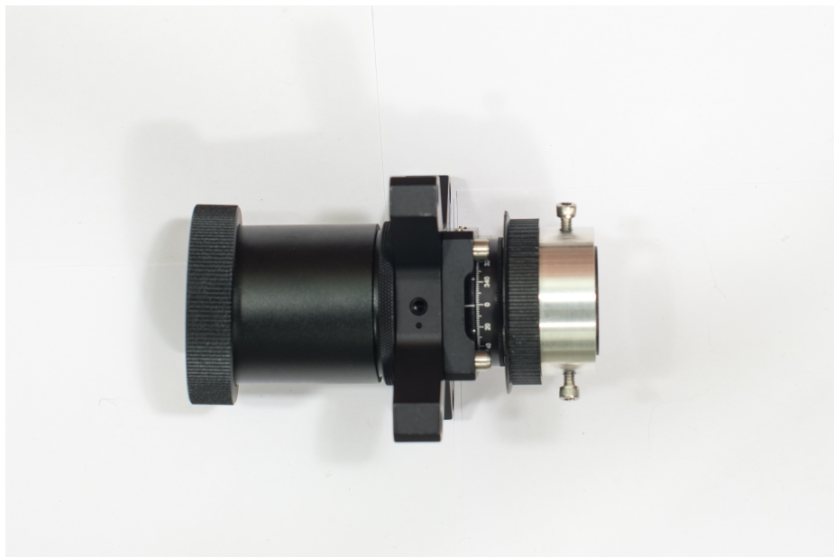
Figure 7: 72 Tooth Pulley, Modified, on Rotation Housing (also shown: SCT to T-Mount, T-Mount to SM1, and 30mm/60mm Cage Plate)
