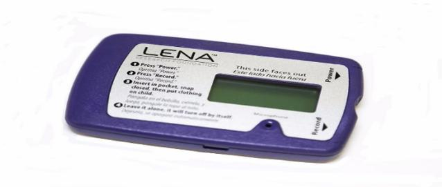
**Step 1:** Press and hold the power button for 3 seconds. This will turn the DLP on. The display screen will read "Sleeping"
