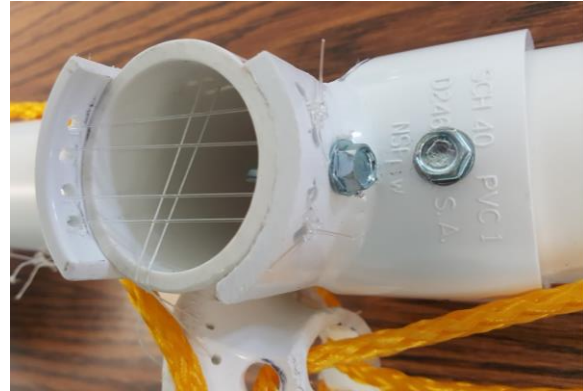
Figure 8 - Screw the DECB as close to the corner as possible, and make sure to screw into the PVC pipe inserted into the VPT and not the empty space below it (also shown in this figure are some of the holes drilled in the DECB, PELPB, and SB; and ligaments).
