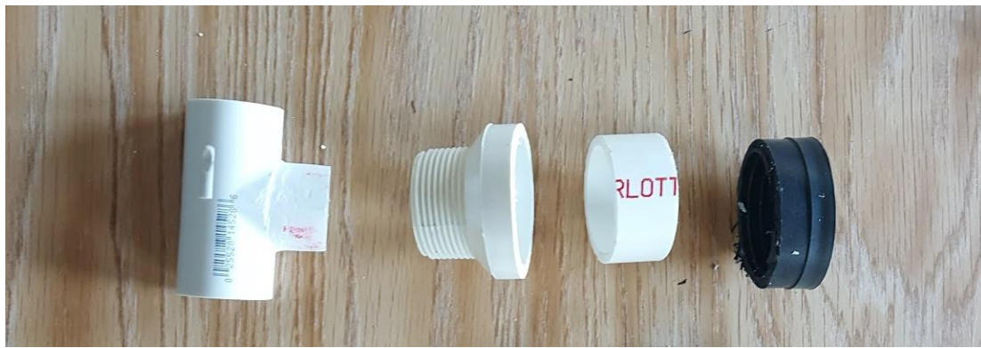
Figure 13: Short pastern bone parts from left to right: ¾” T junction, 1½” → 1¼” male adaptor, 1½” PVC pipe, 1½” quick cap (missing the small length of PVC to go with the T).
