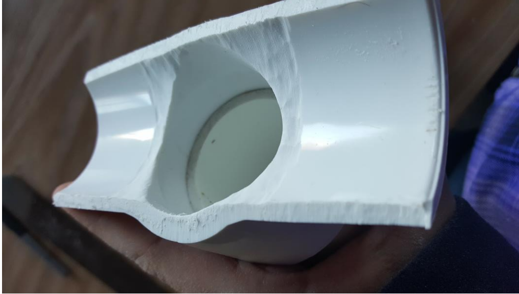
Figure 11: Shows a cut T junction that has the stopping area filed down.
