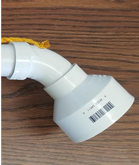
Figure 13 – PVC 1 ½" 30° elbow joint acting as a coffin joint, and a 1 ½" to 3" adapter acting as a hoof.
