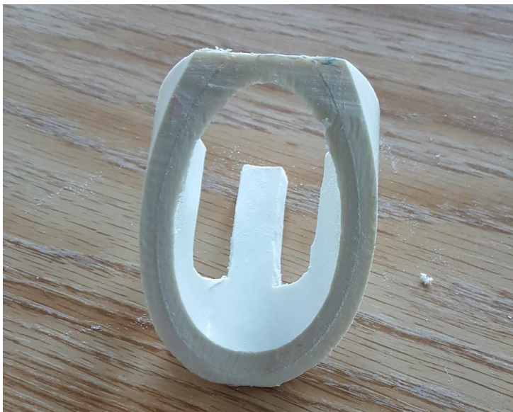
Figure 15: Cut two vertical sections that the T can fit in and file the bottom to be flat.
