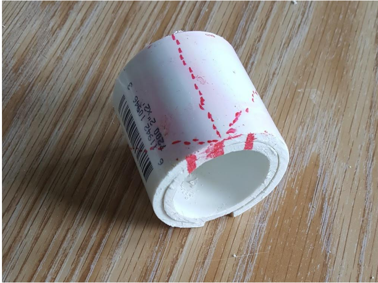
Figure 144: Cut the coffin bone diagonally along both outside dotted lines to make the wedge shape with a flat bottom surface.
