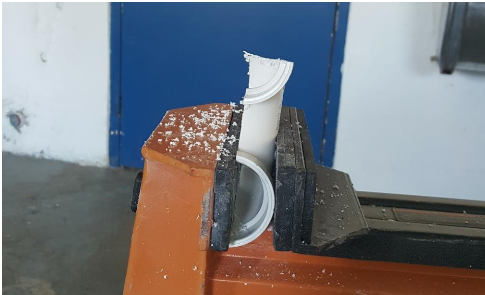
Figure 18: Cut the trap in half length-wise, then each of the ends so that one quarter is left. Only one of the edges is cut off here.
