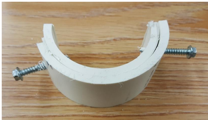
Figure 29: Shows how to screw the collar together so it can be cut and fitted to the model.
