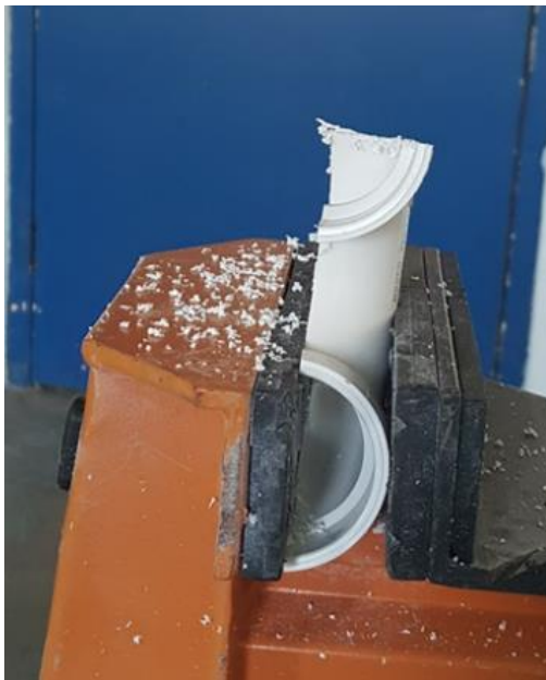
Figure 12 – Cut the trap in half length-wise, then each of the ends so that one quarter is left. Shown here: trap is cut length-wise and only one of the ends is cut.
