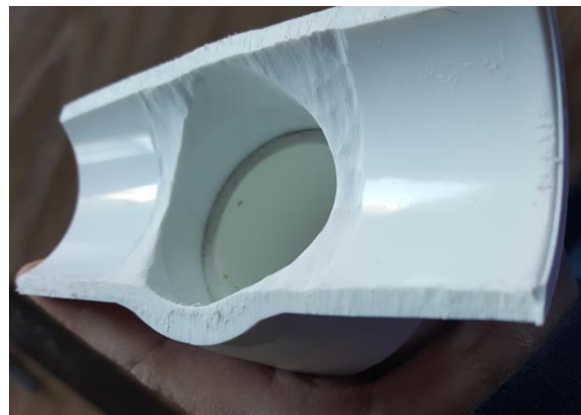
Figure 6 – Grind the lip inside of the HPT flush with the rest of the HPT.
