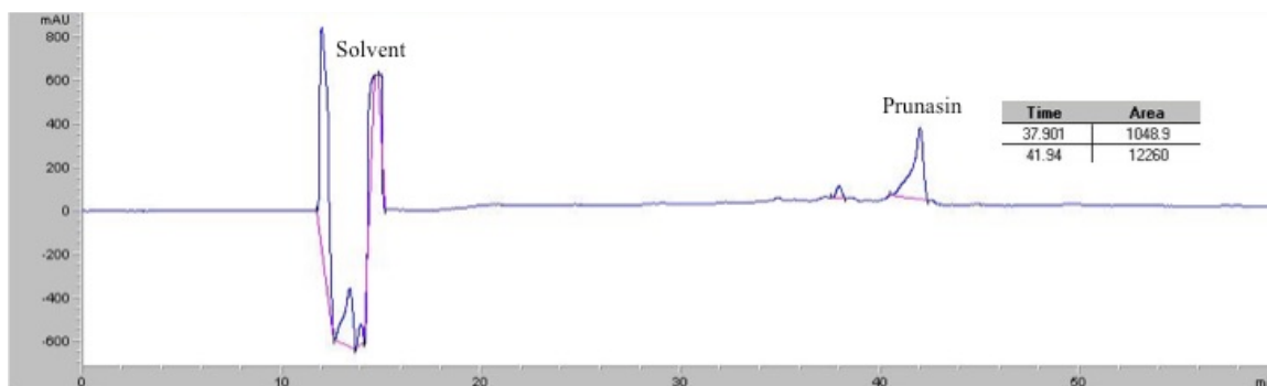
Figure 12: HPLC-UV chromatogram of 0.2 mg/mL prunasin obtained from Sigma-Aldrich. Solvent system B (ultrapure water with 0.05% formic acid and acetonitrile with 0.05% formic acid run at a flow rate of 0.2 mL/min) was used. The peak at 41.94 minutes retention time corresponds to prunasin. Peaks before 20 minutes are due to solvent.
