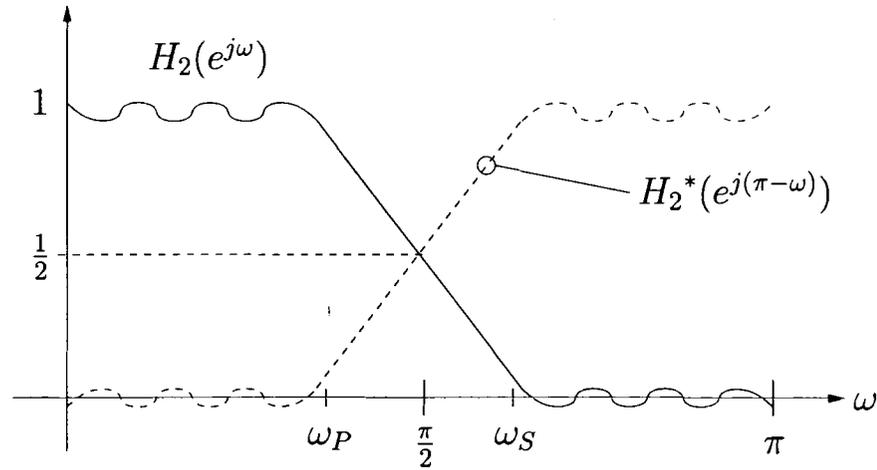
Figure 3.10: Frequency response of a half-band filter
