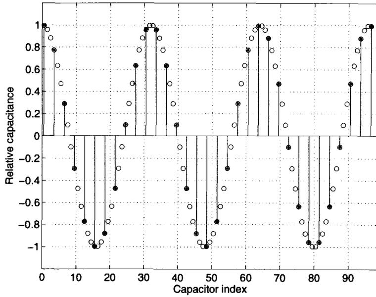
Figure 5.10: Relative modulator capacitance sequence for  $F_m = \frac{3F_s}{32}$
