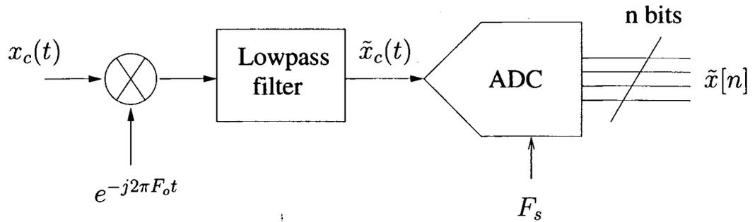
Figure 2.4: Sampling of bandpass signals
