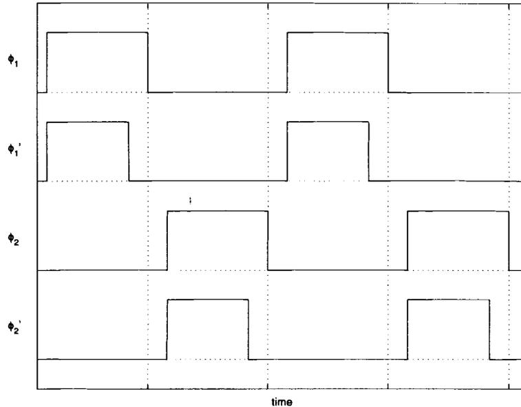
Figure 5.7: Clock phases for  $\Sigma\Delta$  modulator of Figure 5.6
