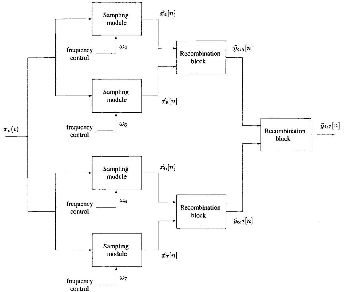
Figure 2.10: Recombination of 4 bands with proposed architecture
