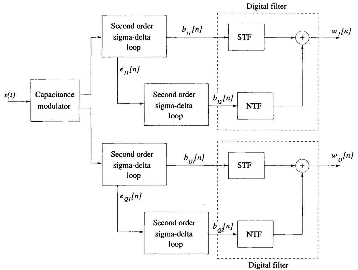
Figure 5.11: Block diagram of frequency selective  $\Sigma\Delta$  ADC
