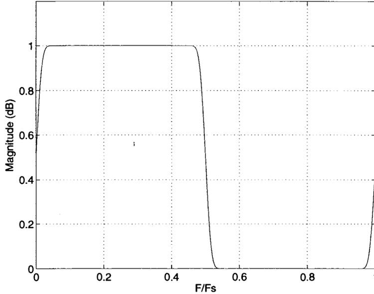
Figure 4.9: Frequency response of a Hilbert transformer
