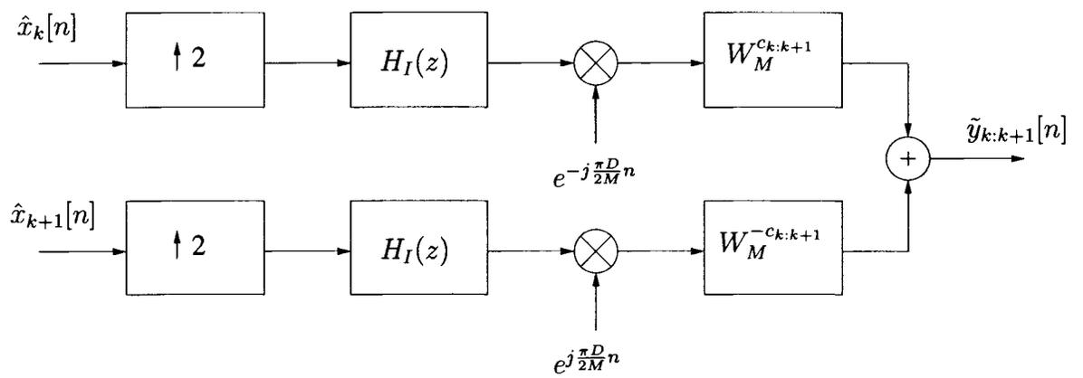
Figure 3.12: Final recombination block design
