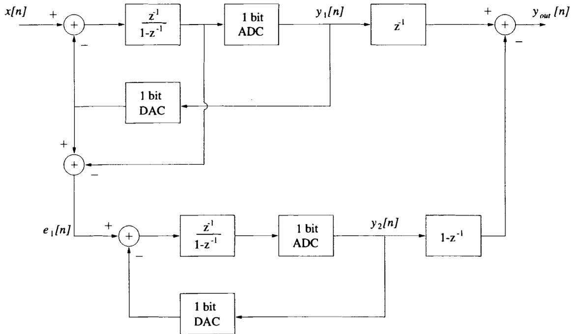
Figure 5.5:  $\Sigma\Delta$  MASH architecture (second order)
