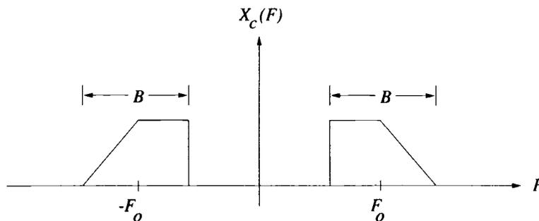
Figure 2.1: Frequency spectrum of a real bandpass signal
