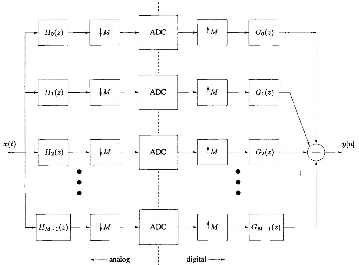
Figure 1.2: M-channel frequency analysis ADC structure
