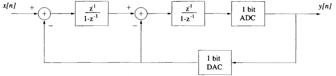
Figure 5.3: Block diagram of a second order  $\Sigma\Delta$  ADC
