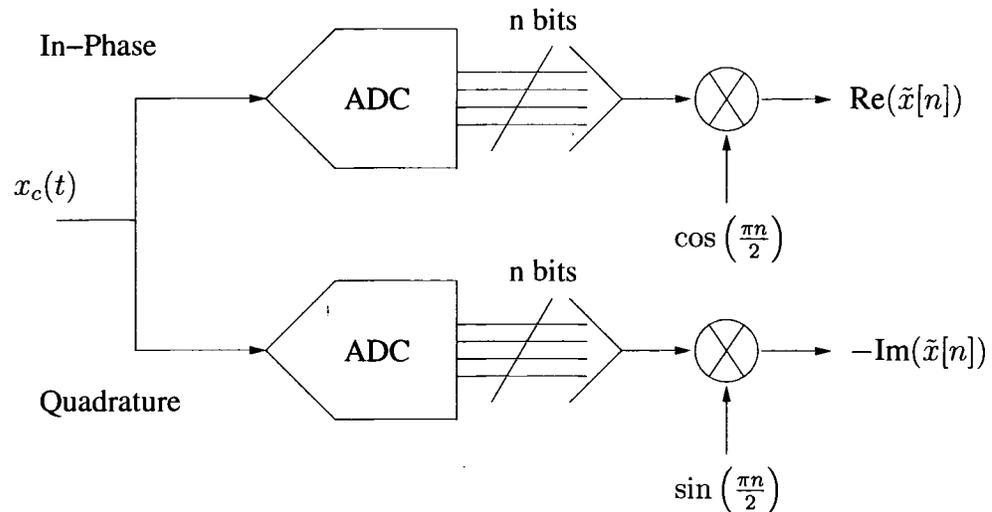
Figure 2.6:  $\frac{F_s}{4}$  subsampling ADC IQ structure
