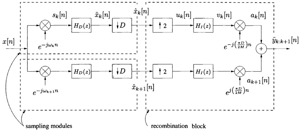
Figure 3.3: Channel recombination for a 2-channel system
