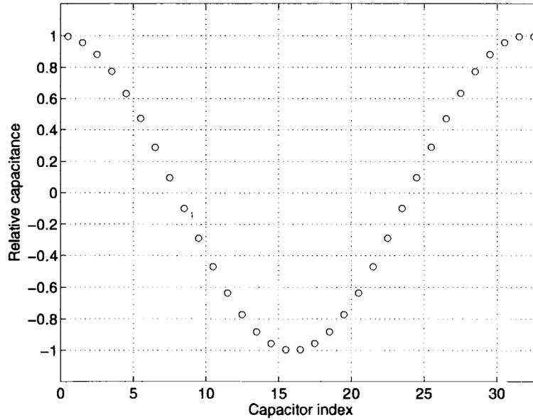
Figure 5.9: Relative modulator capacitance values for OSR of 32
