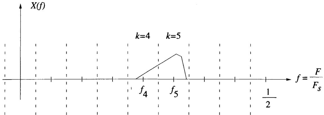
Figure 2.8: Spectrum division for subband quantization
