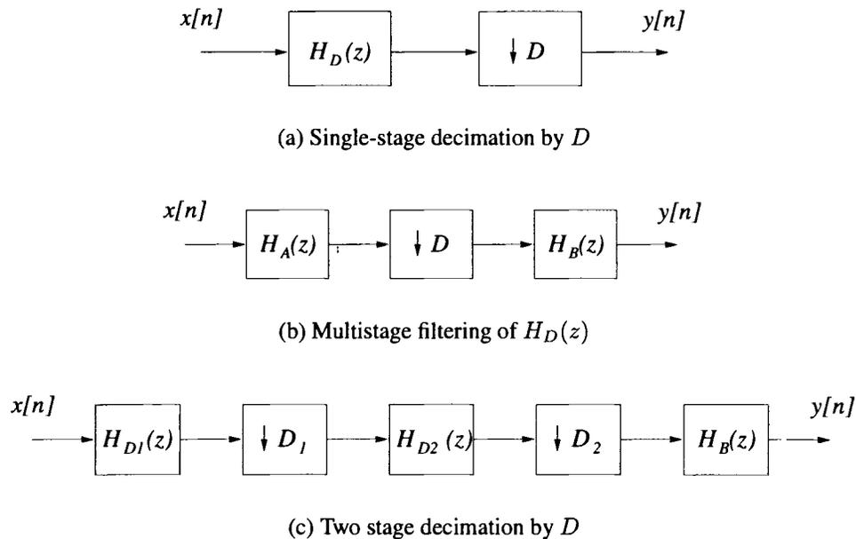
Figure 3.9: Multi-stage decimation and filtering
