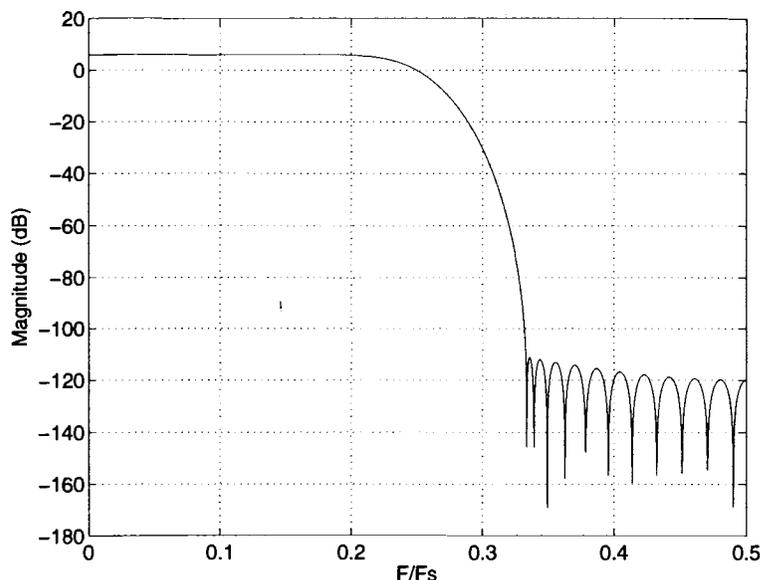
Figure 4.5: Frequency response of interpolation filter  $h_I[n]$
