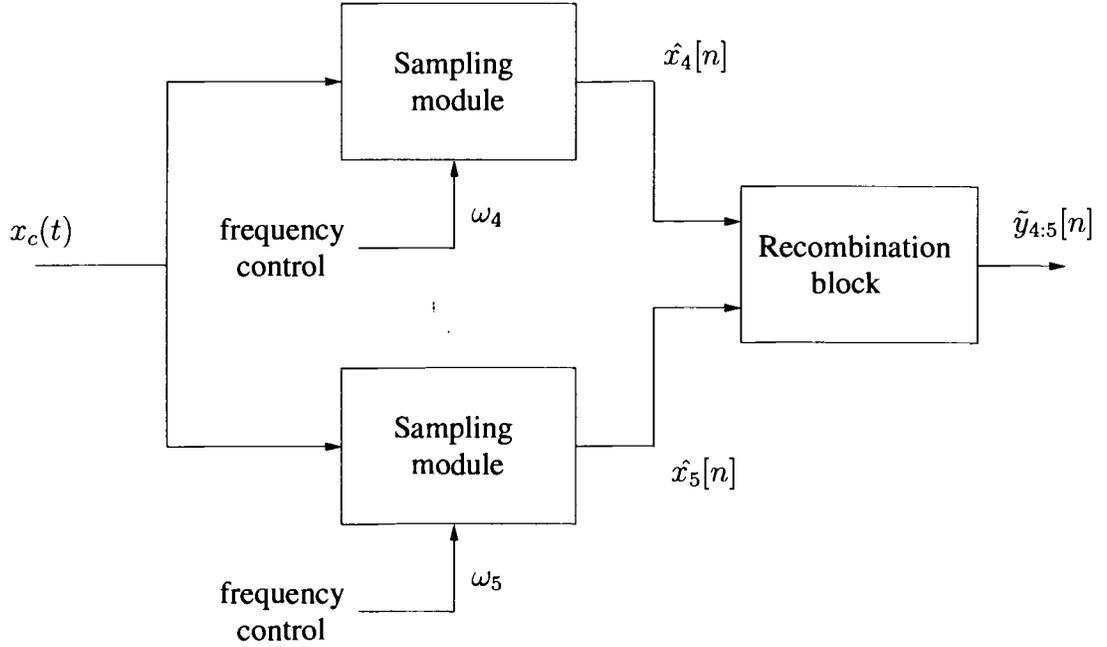
Figure 2.9: Recombination of 2 bands with proposed architecture
