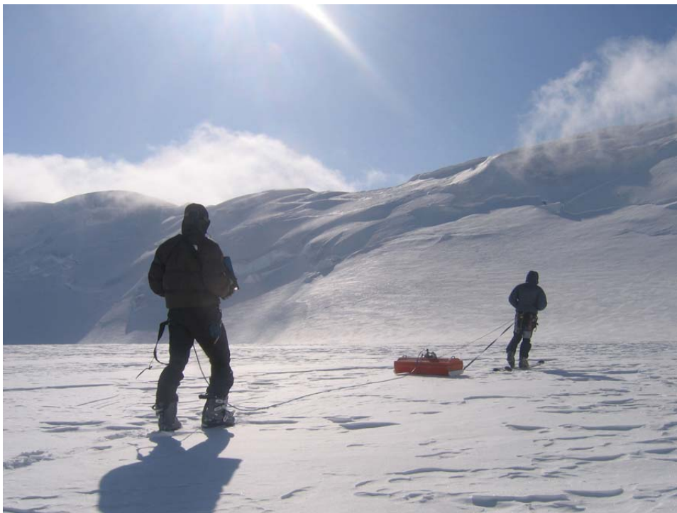
Figure 4. Collecting GPR profiles on the Kahiltna Pass plateau using a GSSI SIR-3000 unit with a 100 MHz antenna.
