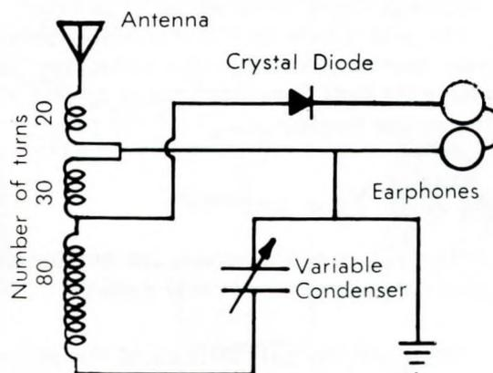
Figure 5—Schematic wiring diagram
