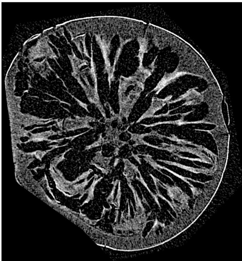
**Figure 6.** *Tomographic cross sectional slice of chitosan bead. Variations in pixel intensity correspond to x-ray absorption, and can thus be correlated with regions of low nano-porosity. Connectivity analysis of pore network can be used to determine pathways through the complex structure.*
