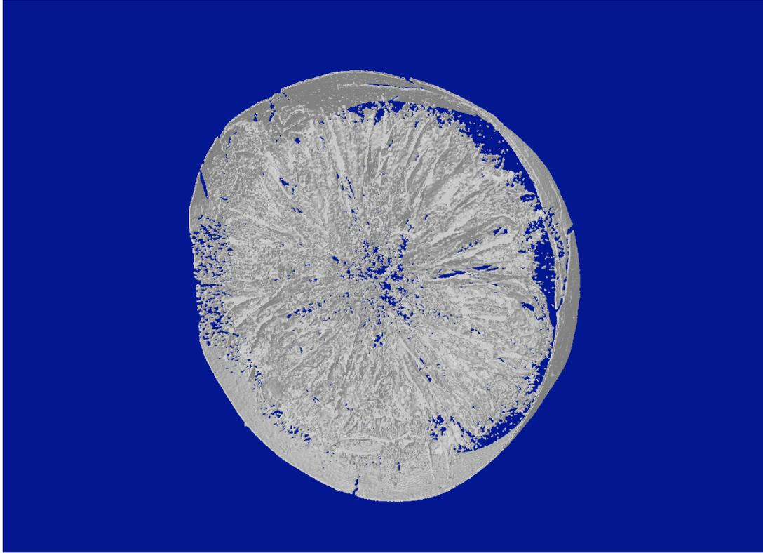
**Figure 7.** 3D rendering of solid phases of chitosan beads. Such data can be used to formulate a computational domain for flow simulations.
