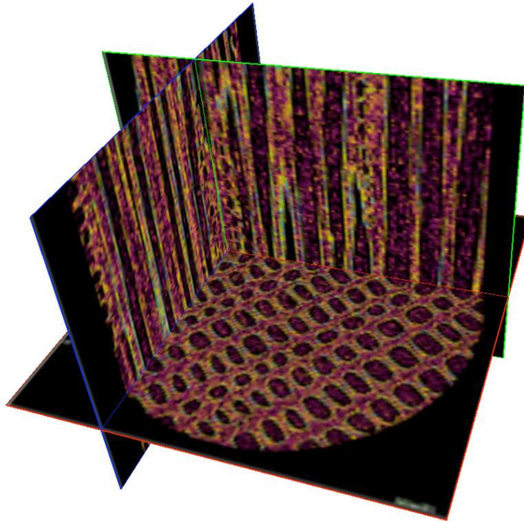
**Figure 4.** 3D sectional representations of a tomographic scan of latewood spruce at 1 micron spatial resolution. The bottom slice shows the transverse cellular structure, while the vertical slices illustrate the longitudinal dimensions of the cells.
