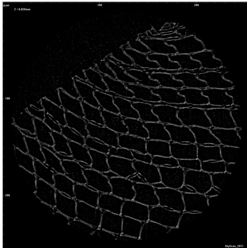
**Figure 3.** Reconstructed slice of earlywood spruce. The 3D spatial resolution approaches 0.5 micron.
