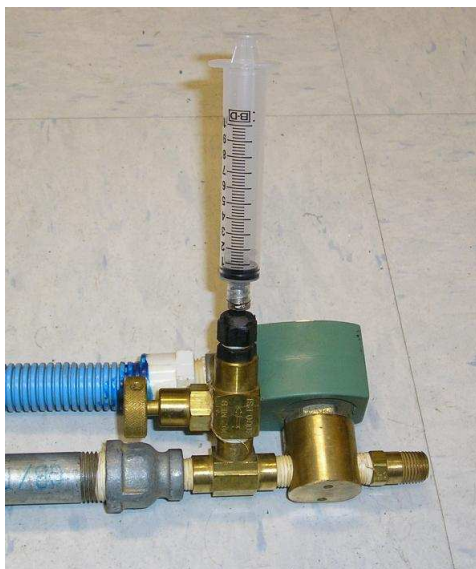
Figure 4.7: A closeup of the discrete interval sampler showing the flow control valve and insertion of a syringe for sample removal.
