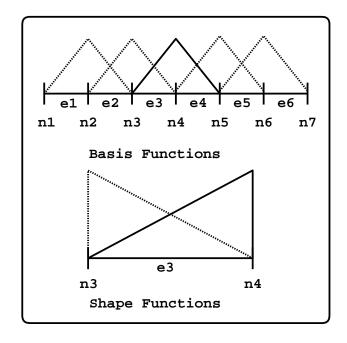
Figure 4.1: Basis and shape functions
