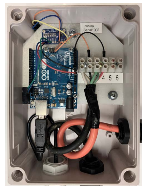
FIGURE 3. Assembly of the precision analog-to-serial converter (PASC) in a water-proof enclosure rated IP66.
