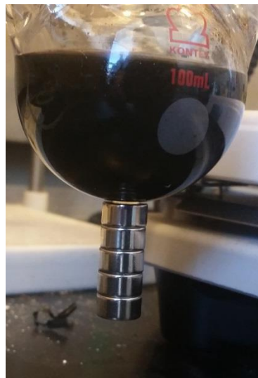
Figure 11: Magnetic Separation of Iron Oxide Nanoparticles from Aqueous Solution
