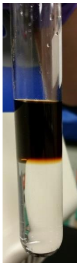
Figure 6: Iron Oxide Nanoparticles Top Layer, PEG Solution Bottom Layer
