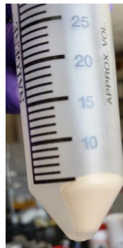
Figure 8: Resulting Pellet from Centrifugation of Phase Transfer Attempt
