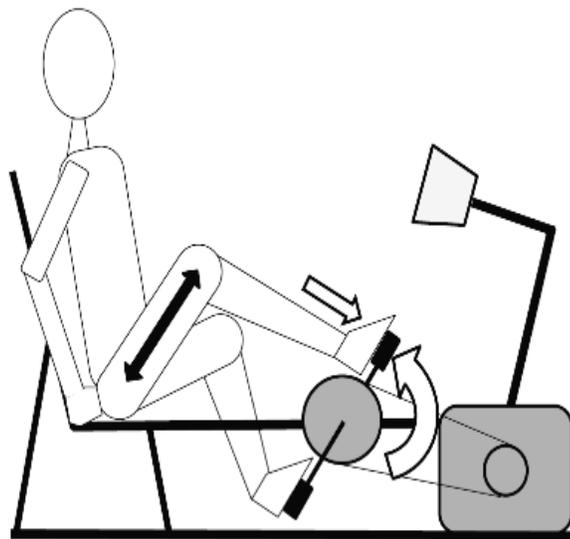
**Figure 1: Eccentric cycle ergometer. As pedals move toward the participant (large white arrow), the participant resists by applying force to the pedals (small white arrow). (Figure adapted from Leong et al., 2013)**
