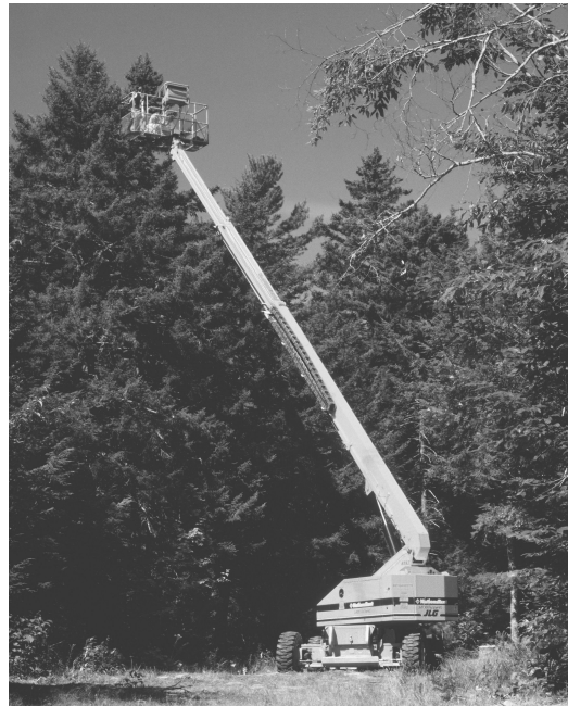
Figure 3. Taking measurements in the grafted crowns of old-growth red spruce trees with a self-propelled hydraulic lift.
