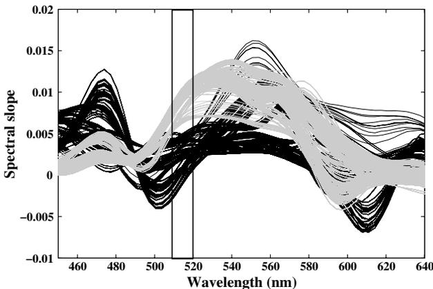
Fig. 4. First derivative spectra of *D. vexillum* (gray) and all other substrates measured (black). The box encloses the unique wavelengths (510–520 nm) that were used in the detection algorithm. Inside the box there is large separation between *D. vexillum* spectra and all other spectra collected.
