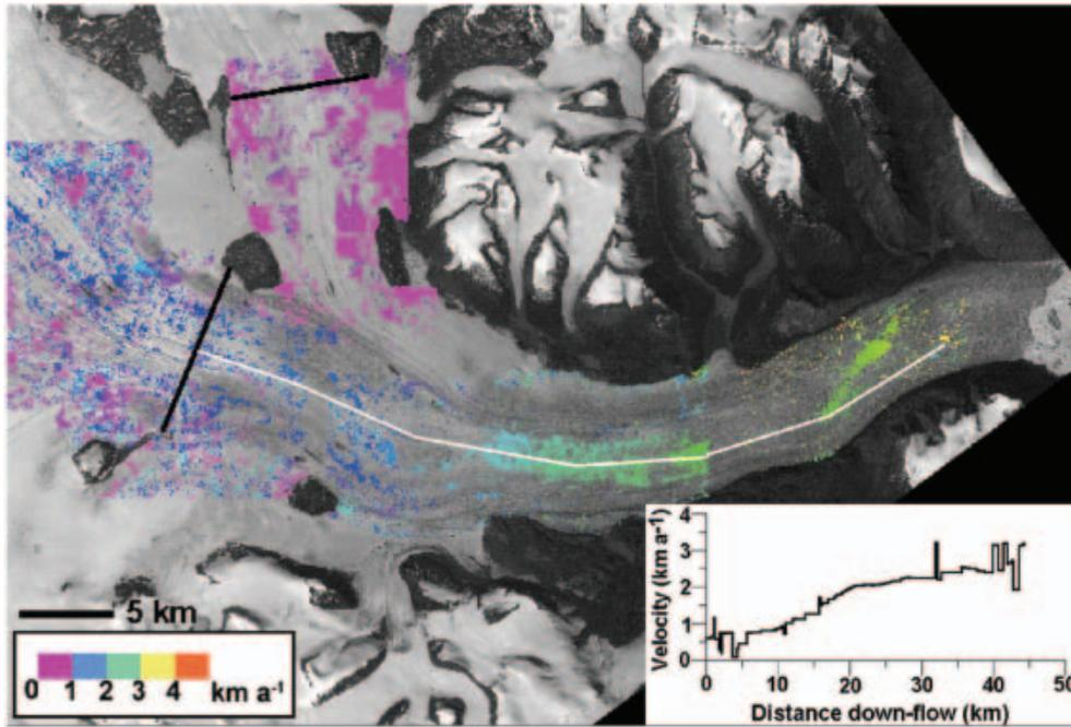
**Fig. 3.** Ice velocities for Daugaard Jensen Gletscher obtained from feature tracking, overlaid on an ASTER image. Black lines represent mass-balance flux gates. The white box shows the region with overlapping velocity measurements from 1968. Inset shows a velocity profile along the thin white line.
