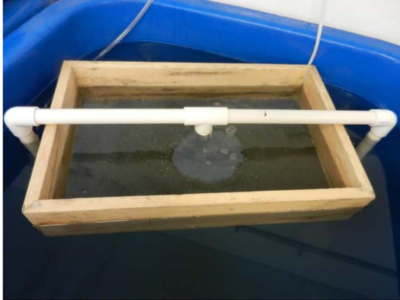
**Figure 5:** Downweller system containing natural sediment.
