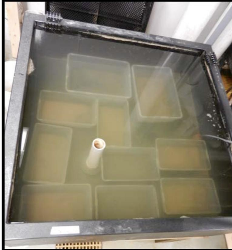
**Figure 6:** Autoclaved tank used in sediment preference experiments. Autoclaved tank used in sediment preference experiments. There were 10 bins containing sediments. The larger bins were split into two sections so that there were a total of 4 “bins” for each sediment type (natural, fine sand, and coarse sand).
