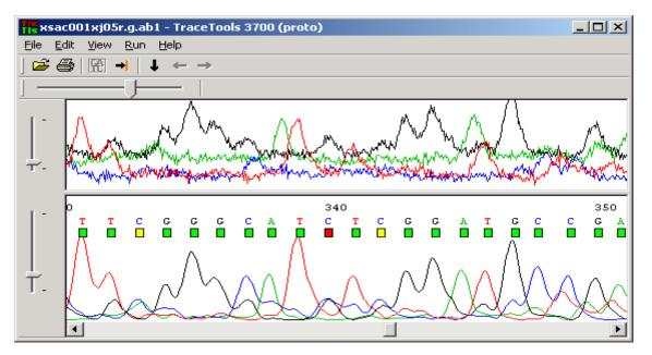
*Figure 2: TraceTools window showing a sequence with bases called and their confidence values indicated by color-coded bars; upper window shows unprocessed data.*
