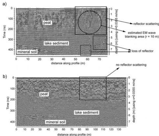
**Figure 4.** Surface GPR profiles collected in Caribou Bog showing (a) reflector scattering and loss of reflectors, and (b) absence of EM shadow zone. Stratigraphic units (in both Figure 4a and Figure 4b) and a circular estimated area affected by EM wave blanking for gas volume evaluation (in Figure 4a) are also shown.
