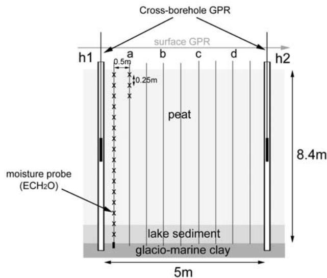
**Figure 1.** Instrumentation setup in the field between boreholes h1 and h2: surface GPR, borehole GPR, and moisture probe with a 1 m offset into the plane of image. Gas samples were collected along lines a, b, c, and d at locations determined by the surface GPR results. Lithological units inferred from direct sampling are also shown.
