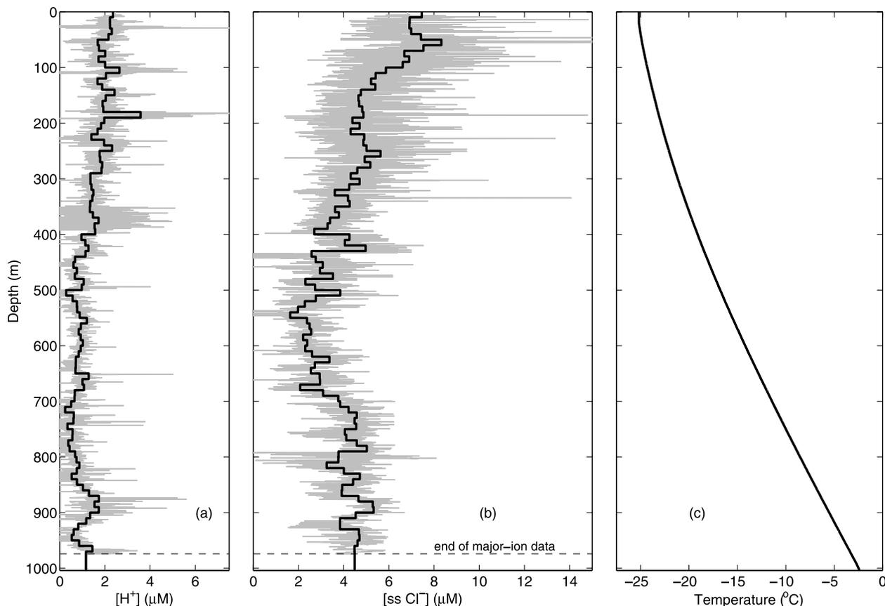
**Figure 2.** Siple Dome ice-core and borehole data used to model attenuation. (a)  $[H^+]$  profile calculated using (8). (b)  $[ss Cl^-]$  profile calculated using (5). For Figures 2a and 2b the concentration axes are at the same scale, the gray lines are the raw profiles, the black lines are the data averaged at 10-m intervals and the horizontal dashed line represents the largest depth for which major-ion data are available (974 m). (c) Measured temperature profile.
