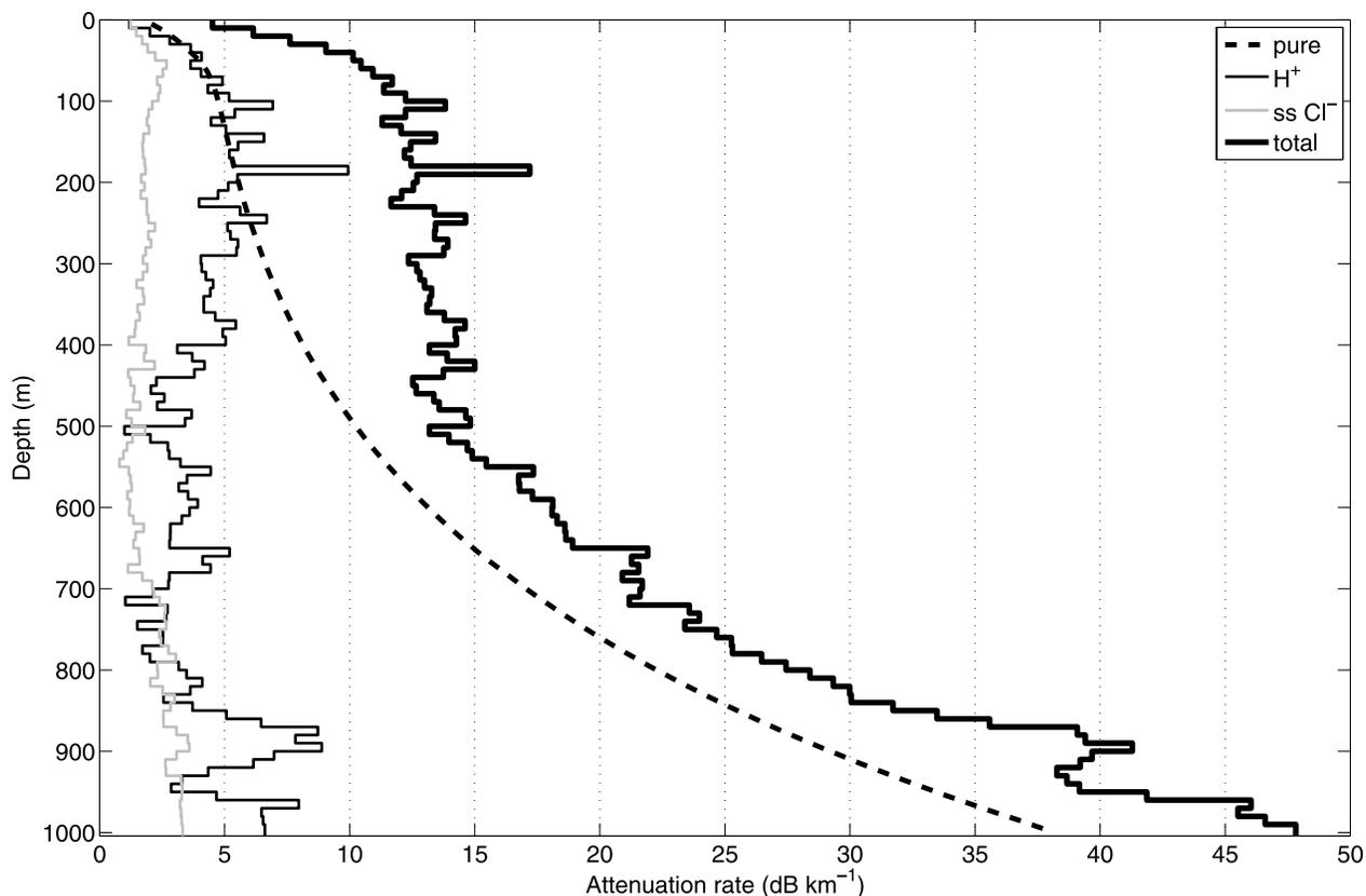
**Figure 3.** Contribution of pure ice,  $H^+$  and  $ss\ Cl^-$  components to the modeled attenuation rate profile ( $N_a$ ) at Siple Dome. At the bed, the depth-averaged modeled attenuation rate ( $N_a^*$ ), calculated from (11), is  $20.0 \pm 5.7\ dB\ km^{-1}$ .
