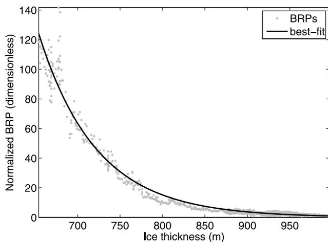
**Figure C1.** Normalized Siple Dome BRPs from traverse data versus ice thickness. Normalized BRP is calculated as the left-hand side of (C1). The solid line is the nonlinear least-squares fit to these data. The traverse data span 54 km both north and south of the ice divide. The best-fit depth-averaged attenuation rate is  $25.3 \pm 1.1$  dB km<sup>-1</sup>; the fraction of explained variance is 0.97.
