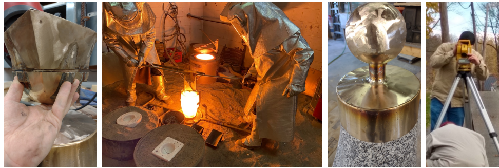
Figure 2 (far left): Polished socket of a custom ball and socket joint. Figure 3: Pouring molten bronze in the UMaine foundry. Figure 4: Polished ball of custom ball and socket joint. Figure 5: Surveying the installation site to find true geographic South.
