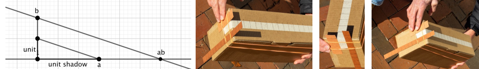
Figure 6 (far left): A multiplication diagram. Figures 7, 8, & 9: Handheld SunRule prototypes showing various products.
