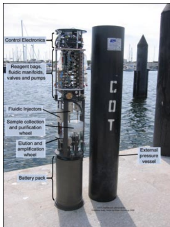
Figure 6. The Autonomous Microbial Genosensor (left) and pressure vessel (right).
