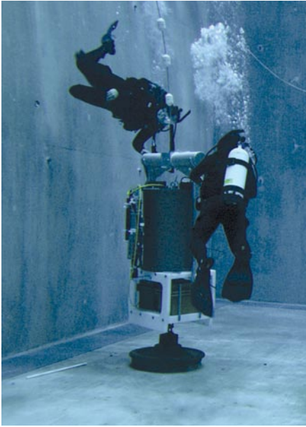
Figure 5. The second-generation Environmental Sample Processor (2G ESP) being tested in a seawater tank ahead of deployment in Monterey Bay. The instrument is moored subsurface and an electromechanical cable provides for communications between a remote station and the ESP's surface buoy. An integral conductivity-temperature-depth (CTD) package is visible at left. The ESP operates on 12-volt rechargeable batteries (at bottom, above the anchor). Photo credit: Todd Walsh, Monterey Bay Aquarium Research Institute
