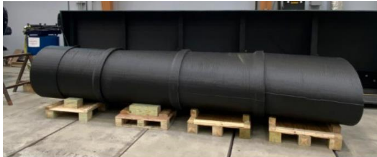
Fig: 3D printed culvert diffuser manufactured at ASCC, UMaine.
