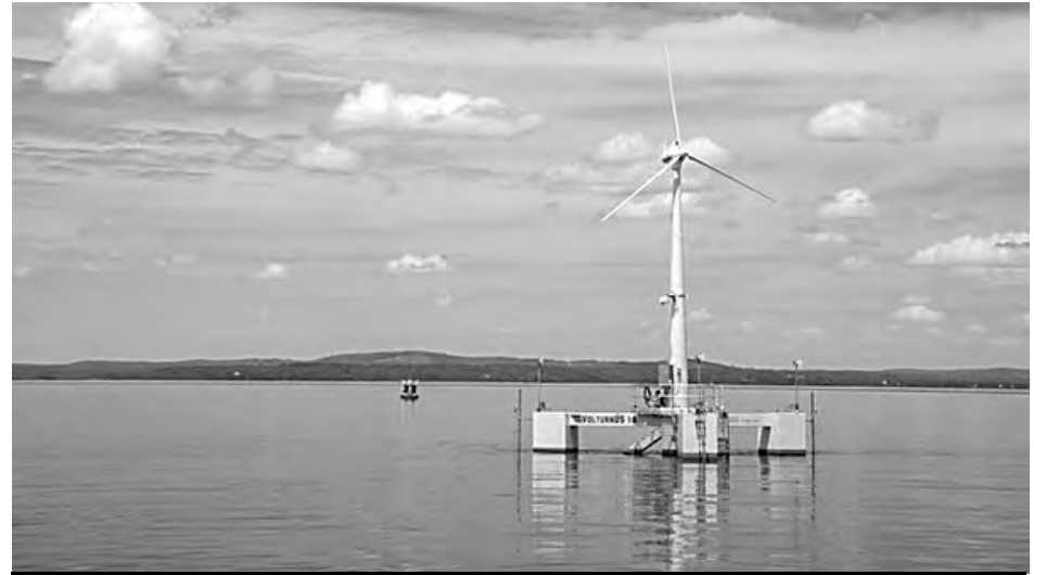
A one-eighth-scale model of Maine Aqua Ventus was tested off Castine. The two turbines planned for the area off Monhegan would be 576 feet tall. University of Maine photo.
