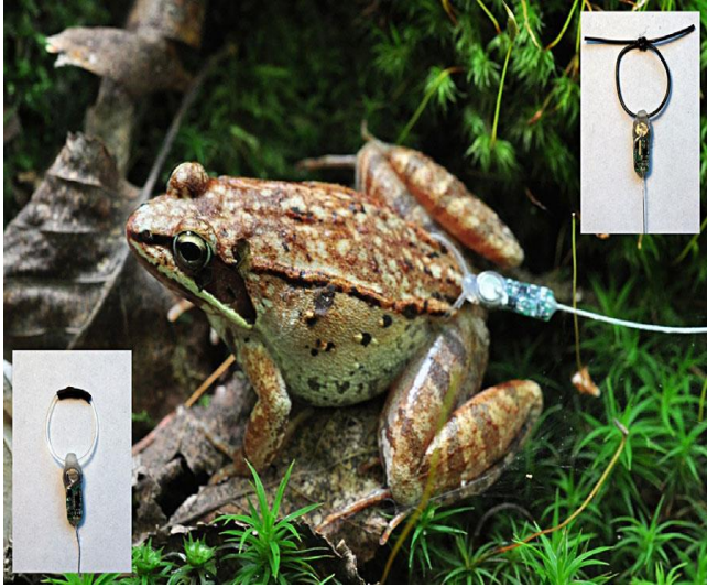
Figure 1. Adult wood frog outfitted with a waistband-mounted radiotransmitter used to monitor movements and habitat use during 2011–2013 in northern Maine, USA. Lower left insert: knotted cord with trimmed ends encased in heat-shrink tubing. Upper right insert: knotted cord with untrimmed ends.
