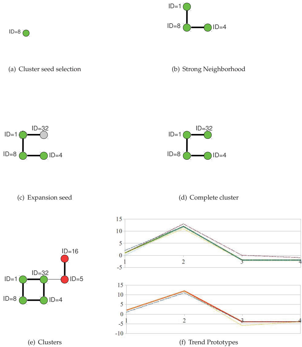
Figure 4: An example of trend cluster discovery by processing the data window shown in Figure 3.
