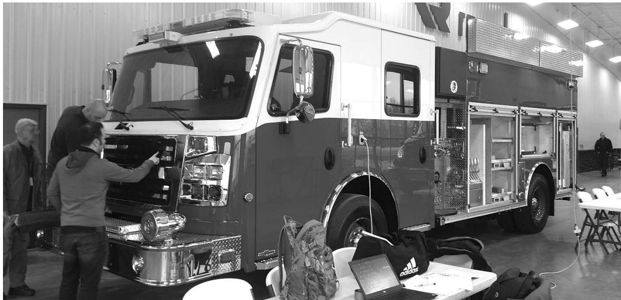
The soon to be delivered Damariscotta Engine 2, a rescue-pumper built by Rosenbauer during a factory final inspection in December of 2018. This apparatus will replace old Engine 2 (1984) and Rescue 5 (1988), and is equipped with a 1,500 gallon per minute pump, 1,000 gallons of water with a custom 5 man cab. The onboard generator will power Jaws of Life and the truck will carry all of the rescue equipment for the Engine Company as well as a full compliment of firefighting tools. Engine 2 will be in service at the beginning of 2019 with a wetdown ceremony to be held in the spring.
