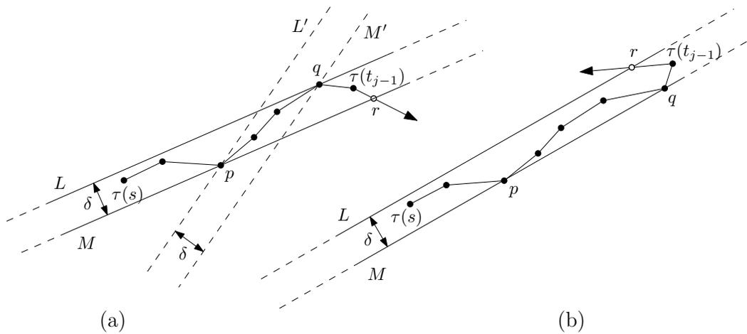
Figure 7: The two cases for the optimal configuration for FURTHEST using a line fitting criterion: (a) The furthest point  $r$  shares a line with  $p$  or  $q$ . (b) The furthest point  $r$  is on the opposite line of  $p$  and  $q$ .
