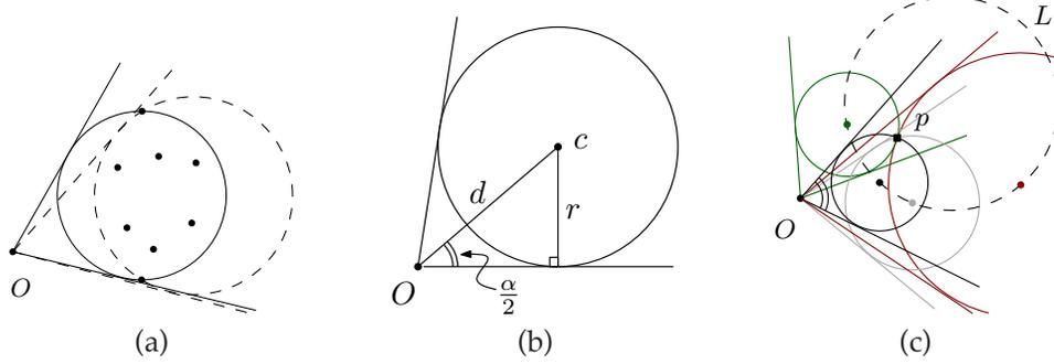
Figure 4: (a) Computing the tangents to the minimum enclosing circle is not guaranteed to give the wedge with smallest angle. (b) The radius  $r$  and the distance  $d$  of the circle center to  $O$  are directly related via  $d \sin(\alpha/2) = r$ . (c) The circles pivoting at a fixed point  $p$  while remaining tangent to an  $\alpha$ -wedge have their center on the circle  $L$ .
