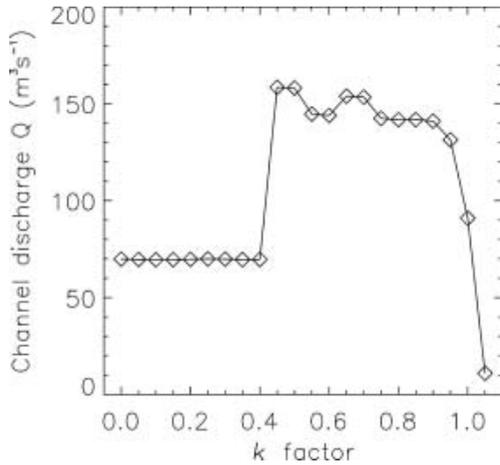
**Fig. 3.** The channel meltwater discharge  $Q$  as a function of the  $k$  factor in Equation (1). The  $k$  factor causes changes in the drainage basin extent, and thus indirectly in the meltwater discharge  $Q$ .
