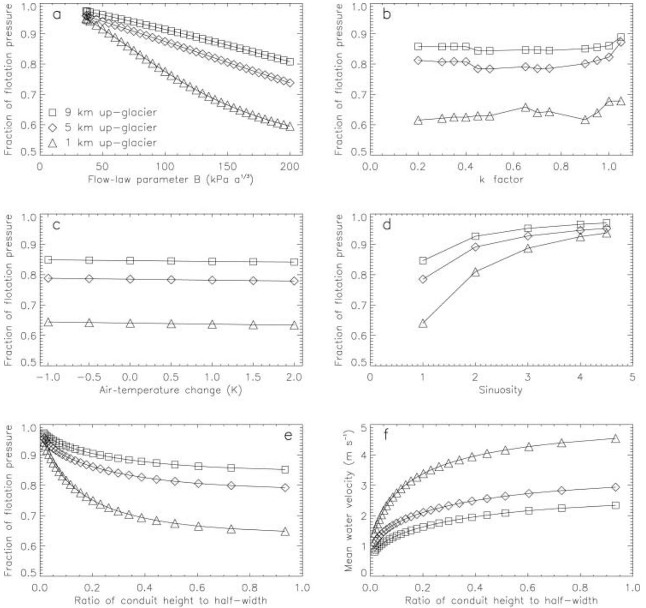
**Fig. 5.** (a–e) The influence of various parameters on the water pressure at three distances from the ice margin in a selected subglacial channel. The legend in (a) is valid for all plots. See text for a detailed explanation of the plots. (f) Calculated mean water speed in the subglacial channel as a function of channel geometry.
