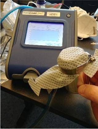
Figure 3: Test material sealed to chamber
