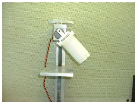
Figure 10 - Photograph of the dipping apparatus used to deposit silica sols on alumina and single crystal silicon substrates.
