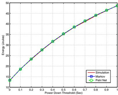
Figure 7. Energy Estimates for Power\_Up\_Delay = 0.001 Seconds
