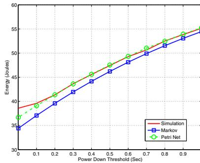
Figure 8. Energy Estimates for Power\_Up\_Delay = 0.3 Seconds
