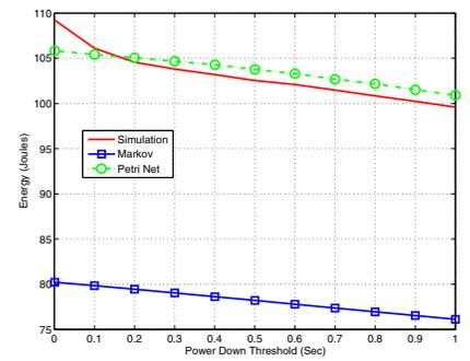
Figure 9. Energy Estimates for Power\_Up\_Delay = 10 Seconds
