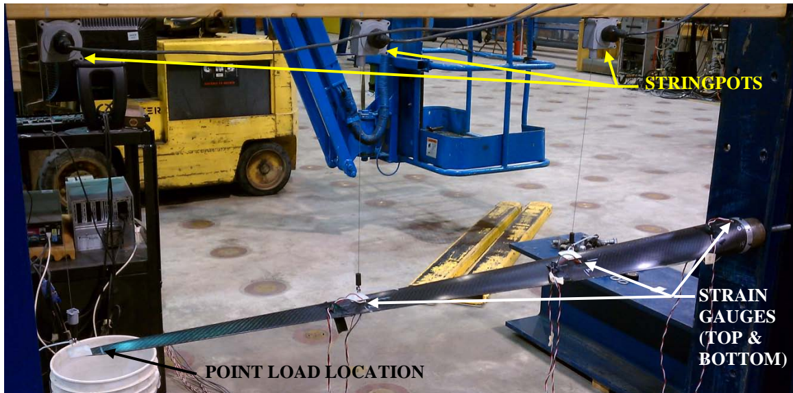
Figure 4.5. Cantilever bending test set up for 1/50th scale model blade.
