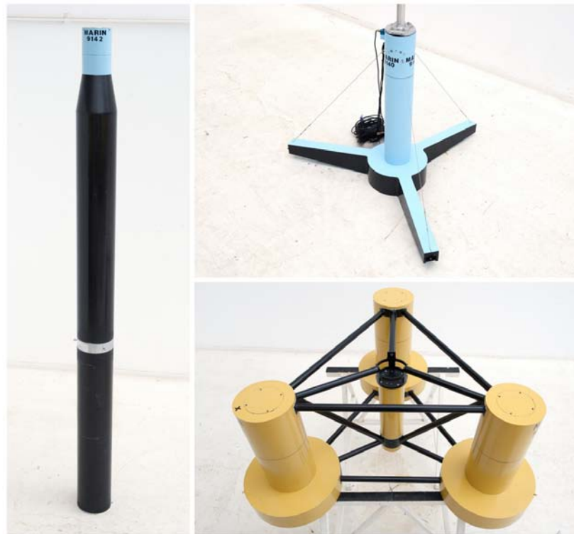
Figure 1.3. 1/50 th scale floating platforms tested at MARIN. Clockwise from left: OC3 Hywind spar-buoy (left), TLP (top right), and semi-submersible (bottom right).
