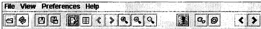
Figure 5.7. The menu bar and toolbar of the prototype application. From left to right: open, reopen, save, save as, show sketch properties, show relation matrix, highlight previous region, highlight next region, zoom in, zoom out, zoom to extent, extract regions on/off, set modules, fill gaps on/off, show previous sketch in process tab, show next sketch in process tab.
