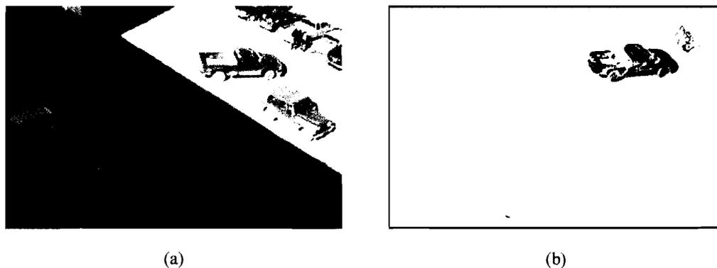
Figure 4.5: (a) original video containing a few moving objects (red truck and two people); (b) raw AFD output of the original frame (black border artificially added to delimit AFD frame)
