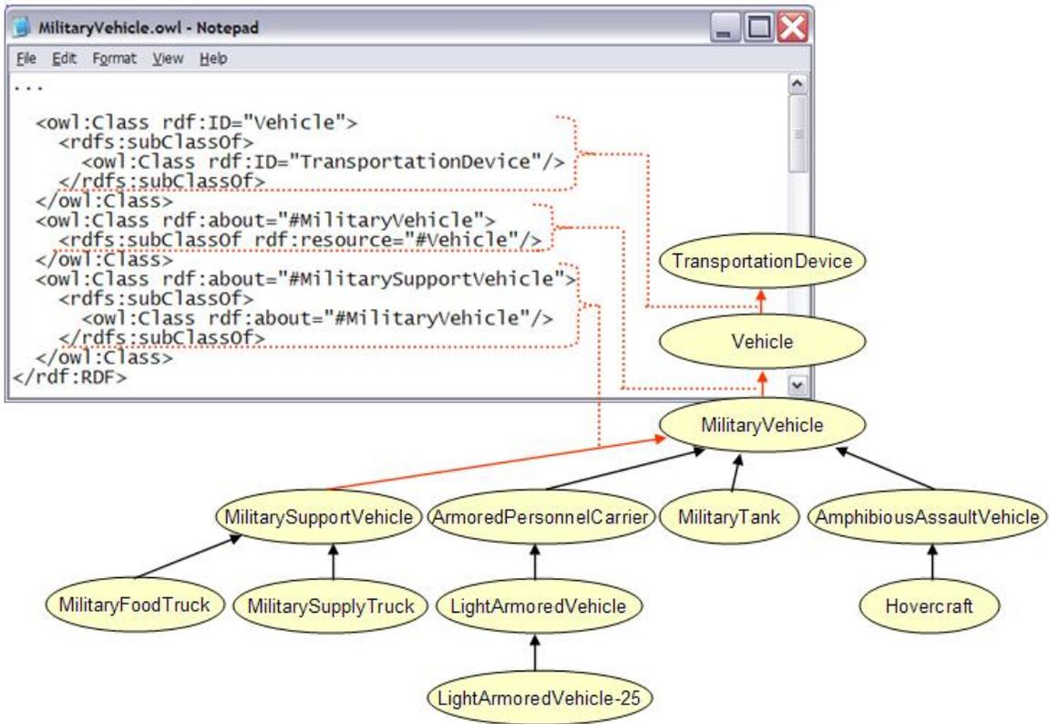
Figure 4.1. An RDF representation for ontology class hierarchy
