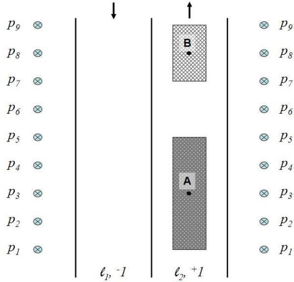
Figure 5.2. Modeling vehicle movement at time  $t$ , where  $isBehind(a,b,T)$  and  $inFrontOf(b,a,T)$
