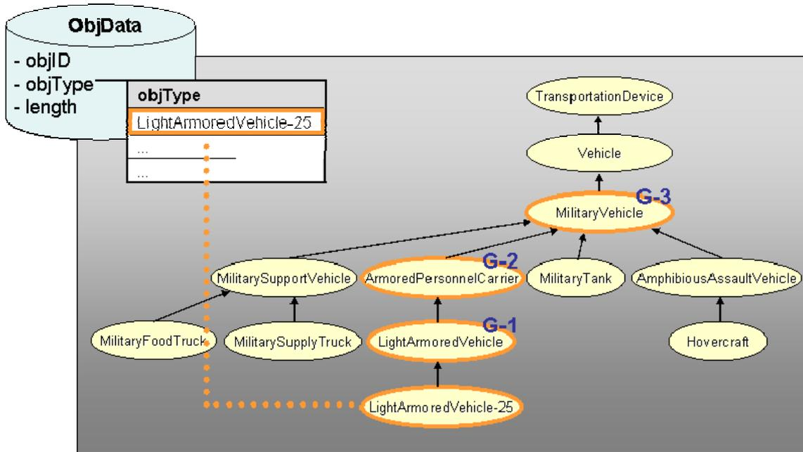
Figure 5.10. Generalization of the ontology class *lightarmoredvehicle-25* where the 1<sup>st</sup> generalization = G-1, 2<sup>nd</sup> generalization = G-2 and 3<sup>rd</sup> generalization = G-3.
