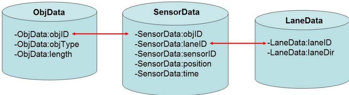
Figure 3.3. Database structure for storing moving object data.
