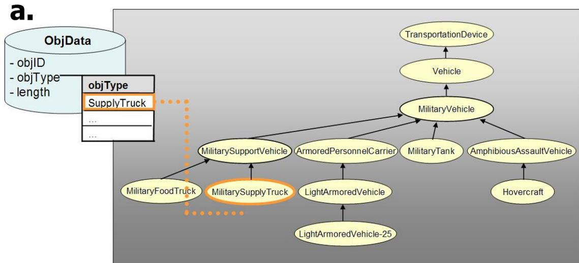
Figure 2.4. Linking between a database (a) and an ontology (b) to share information
