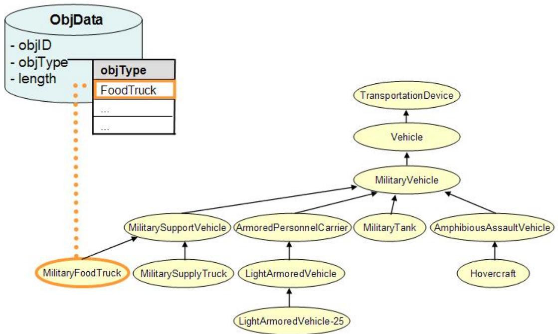
Figure 4.2. Linking a geospatial database with the *military transportation device* ontology.
