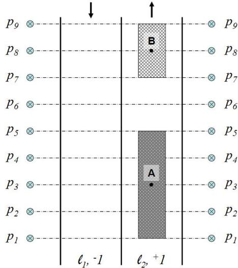
Figure 5.4. Vehicle *A* is behind vehicle *B* with *laneDir* = +1
