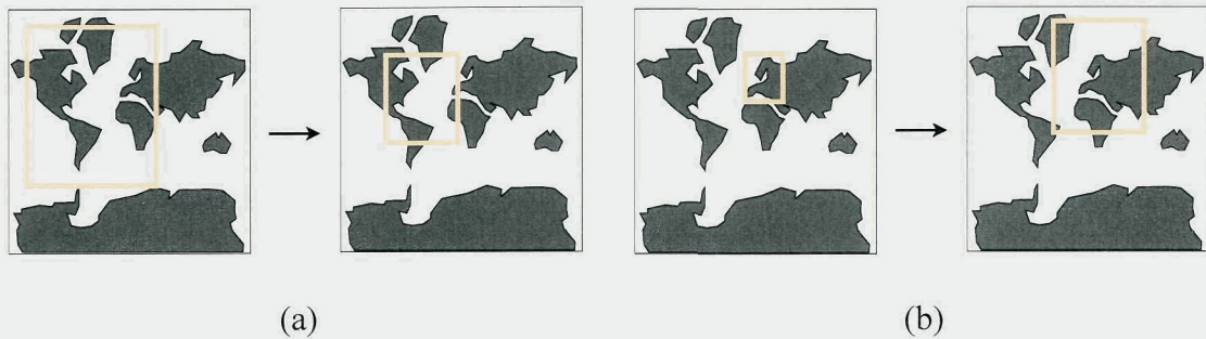
Figure 3.7: Zoom operations. V represented as highlighted rectangle: (a) zoom in and (b) zoom out.
