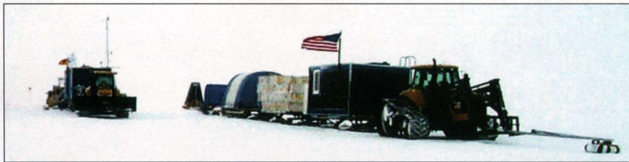
Fig. 2. U.S. ITASE traverse tractors and sleds are shown; crevasse detection equipment is mounted on lead tractor. Sleds contain berthing, kitchen, fuel drums, scientific equipment, and ice cores.
