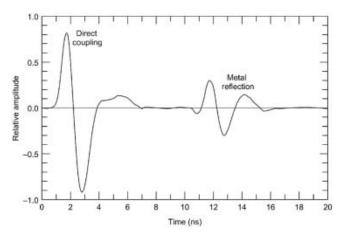
**Fig. 2.** The 400 MHz antenna waveforms. The amplitudes of the direct coupling between transmitter and receiver antennas and the metal reflection are cross-references used to measure reflectivity values for the firn horizons. The +-+ phase polarity sequence (red-blue-red in the profiles) to the major half-cycles of the reflection is the inverse of that of the wavelet transmitted into the firn.
