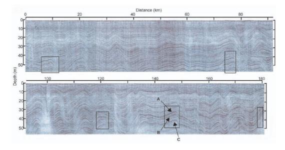
**Fig. 3.** Profile of transect I, from BSC going west. The boxes enclose the same set of three horizons, A–C, at least two of which were tracked along all transects in Figure 1. The depth scale is adjusted to the average relative dielectric permittivity,  $\varepsilon$  = 2.4, for the depth of 56 m. The vertical exaggeration is 348:1. The stronger distortion occurs at 75–110 and 150–180 km, where the transect traversed a series of hills. Cores have been obtained at 0, 90 and 181 km.
