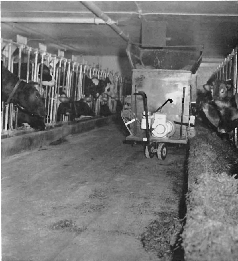
FIGURE 1. Self propelled, self unloading cart for mechanized silage feeding in stanchion barns.
