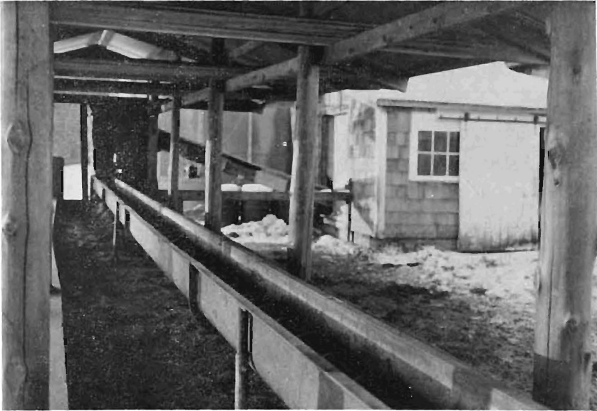
FIGURE 6. Auger feeding of haylage. Note the elevator in the background which brings haylage onto the auger from a bottom unloaded silo.
