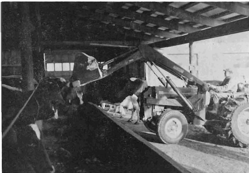
FIGURE 9. Feeding silage directly to bunks with a tractor-bucket. An excellent method when used with a horizontal silo located near the feeding area.
