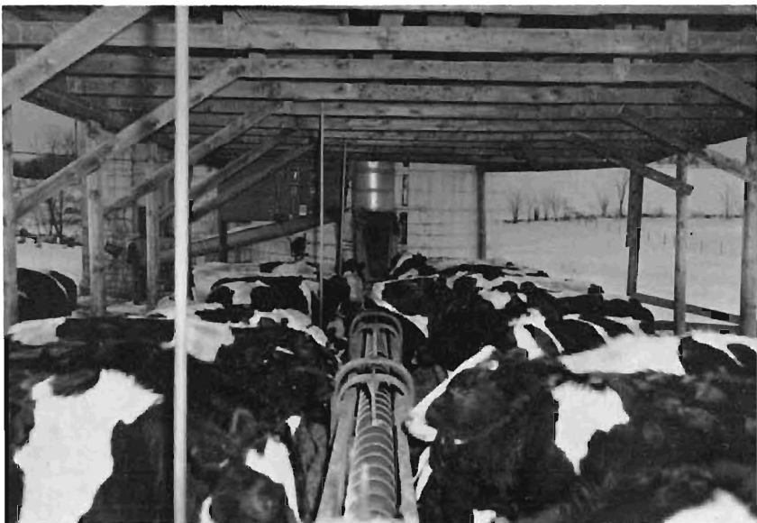
FIGURE 7. Auger feeding of silage. Silage is removed by an unloader in the top of the silo and moved by gravity directly to auger. Note the silage chute in the background.
