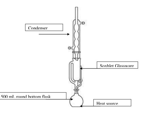
Figure 5: Schematic of a Soxhlet apparatus (Grainger Industrial Supply)
