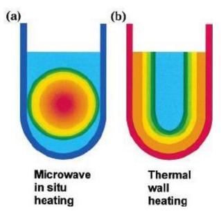
Figure 2. (a) Schematic illustration of microwave *in situ* heating. The heat is transferred directly into reaction mixture. (b) Classic wall heating. The heat energy must be transferred via the vessel wall. The darkest color indicates the most intense heat. (Larhed *et al.* 2002).
