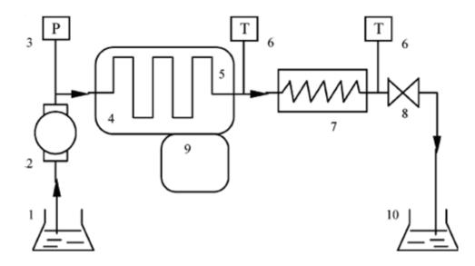
Figure 3 is a schematic diagram of the CMR. 1, reaction mixture; 2,metering pump; 3, pressure transducer; 4, microwave cavity;, 5, reaction coil; 6, temperature sensor; 7, heat exchanger; 8, pressure regulator; 9, microprocessor controller; and 10, product vessel. (Roberts and Strauss 2005).
