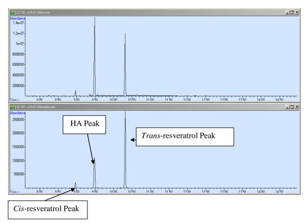
Figure 8: GC chromatogram of the  $40 \,\mu\text{g/mL}$  concentration resveratrol standard. The bottom chromatogram is the selected ion chromatogram.
