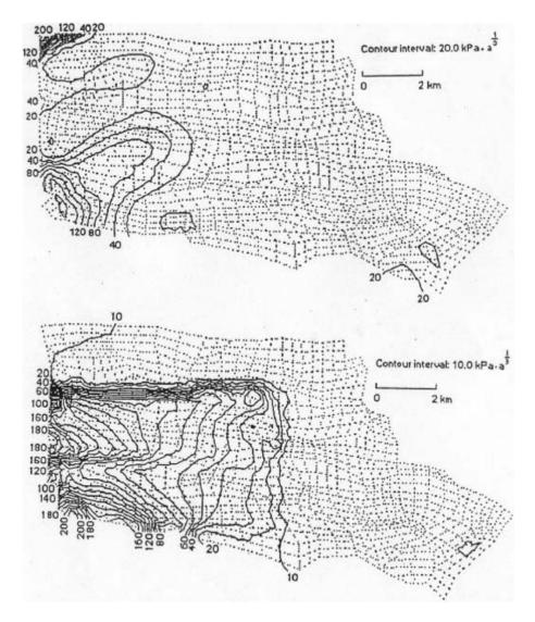
Fig. 6. Results from calculating B using the control method and measured velocities for n=3 and plane stress. Top: results from a Fourier series expansion in 52 terms contoured every 20 kPa a<sup>1/3</sup>. Bottom: results from a Walsh series expansion in 12 terms contoured every 10 kPa a<sup>1/3</sup>.
