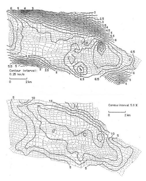
**Fig. 5.** Comparison of measured velocities in the refined finite-element mesh with velocities calculated for plane stress,  $B = 180 \,\text{kPa} \,\text{a}^{1/3}$ , and n = 3 in the Glen (1958) flow law of ice. Top: measured velocities contoured every 0.25 km a<sup>-1</sup>. Bottom: per cent difference between measured and calculated velocities contoured every 5%.
