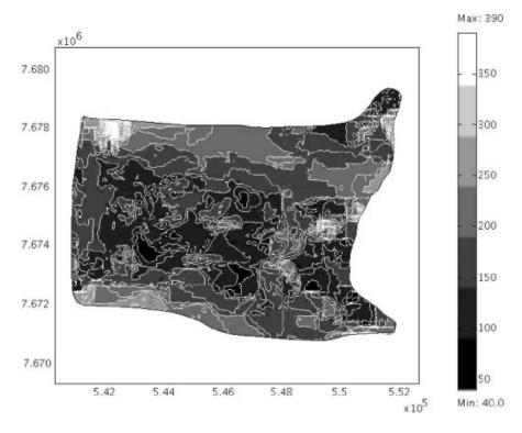
**Fig. 11.** The effective stress field on the floating portion of Jakobshavn Isbræ, computed using measured velocities and their derivatives. Units of kPa. Contours are spaced at 25 kPa. Large fluctuations in the stress are seen propagating across the ice in the transverse direction, possibly indicating force chains, which resist longitudinal flow.
