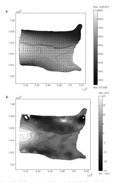
**Fig. 9.** Results of the ice shelf with Zipper experiment. (a) Computed velocity field. Gray scale indicates magnitude of velocity; scaled arrows show direction. Contours are at 250 m a<sup>-1</sup> intervals. Feature modeled as the Zipper is shown with black line. (b) Percentage differences between computed and measured velocities for the floating portion of Jakobshavn Isbræ. Contours are at 5% intervals.
