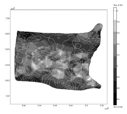
**Fig. 7.** Calculated base 10 log of effective viscosities  $\eta$  for  $\bar{B}=180$  kPa  $a^{-1/3}$ . Values are obtained from velocity data by using finite-element basis functions to compute ice-velocity derivatives for Equation (7). Contours show ice thickness at 25 m intervals.
