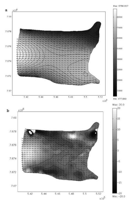
**Fig. 8.** Results of the uncrevassed ice-shelf experiment. (a) Computed velocity field. Gray scale indicates magnitude of velocity; scaled arrows show direction. Contours are at 250 m a<sup>-1</sup> intervals. (b) Percentage difference between computed and measured velocities for the floating portion of Jakobshavn Isbræ. Contours are at 5% intervals.
