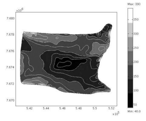
**Fig. 12.** The effective stress field on the floating portion of Jakobshavn Isbræ computed from results of the uncrevassed ice-shelf experiment. Units are kPa. Contours are spaced at 25 kPa. There are no high-stress regions that propagate transversely across this ice, indicating that continuum mechanics fails to capture all the dynamics of this system.
