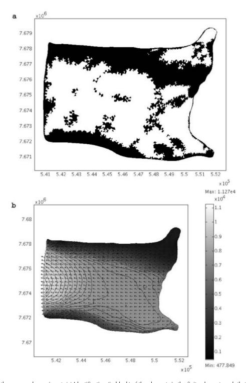
**Fig. 10.** Results of the crevassed experiment. (a) Identification (in black) of the elements in the finite-element mesh that are assumed to be fragmented, and are therefore given a linear rheology in the fragmented ice-shelf experiment. (b) Results of the fragmented ice-shelf experiment. Gray scale indicates magnitude of velocity; scaled arrows show direction. Contours are at 250 m a<sup>-1</sup> intervals.
