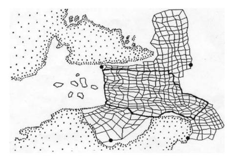
Fig. 4. The finite-element mesh used for modeling Jakobshavn Isbræ. Elements within the bold border are for floating ice, with each finite-element domain subdivided into four smaller domains for this study.
