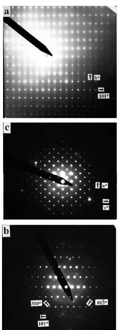
FIG. 3. (a) Electron diffraction pattern with beam parallel to  $[10\bar{1}]$ . Overexposed near origin to show up the diffuse streaks. Långban sample. (b) Diffraction pattern with beam parallel to  $[\bar{1}31]$ . Dara-i-Pioz sample. (c) Diffraction pattern with beam parallel to [010]. Långban sample. Camera length was 1200 mm for all diffraction patterns.
