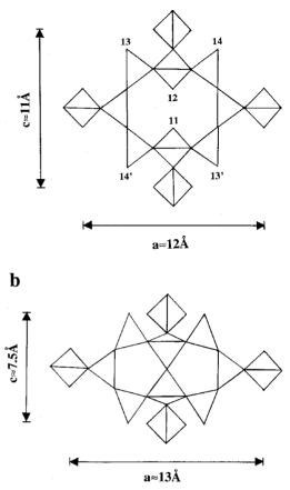
FIG. 1. Comparison of portions of (*a*) the hyalotekite framework and (*b*) corresponding portion of the scapolite structure. Both structures are idealized and have their maximum possible *I4/mmm* symmetry. Nonbridging oxygens in (*a*) are numbered according to the scheme of Moore *et al.* (1982).
