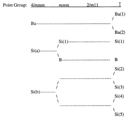
FIG. 2. Splitting of hyalotekite atom sites as the symmetry is lowered stepwise from I4/mmm to  $I\overline{1}$ . (a) cations, (b) (opposite) anions. Note: Pb site splits in a similar fashion to the Ba site. The Ca and F sites do not split.
