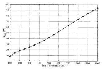
Fig. 7. Maximum crevasse penetration as a function of ice thickness for zero back stress.
