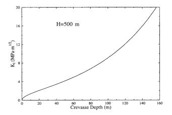
Fig. 8. Stress intensity factor for a basal crevasse as a function of penetration depth, measured from the base of the ice, for  $\sigma_c = 0$ . Overburden stress on its own is insufficient to pinch shut a crack once growth is initiated, because  $K_1$  increases with crevasse depth without bound.
