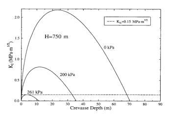
(b) Fig. 5. Stress intensity factor as a function of crevasse depth for a range of back stresses.
