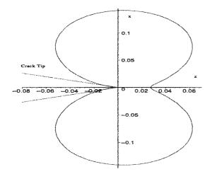
Fig. A1. Polar plot of the plastic zone  $r_p$ , measured in metres, for plane strain conditions.
