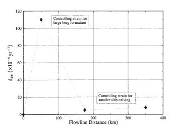
**Fig. 12.** Calculated strain rates along the Byrd Glacier flowband onto the Ross Ice Shelf. Larger strain rates farther upstream may be the controlling mechanism for large scale iceberg formation, while smaller strains nearer the calving front may control the smaller and more frequent calving events.
