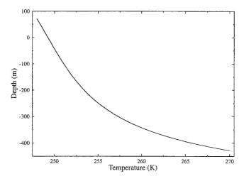
**Fig. 4.** The temperature profile as a function of depth for a glacier of thickness 500 m experiencing basal melting. Surface temperature is -25°C and basal temperature is -3°C.
