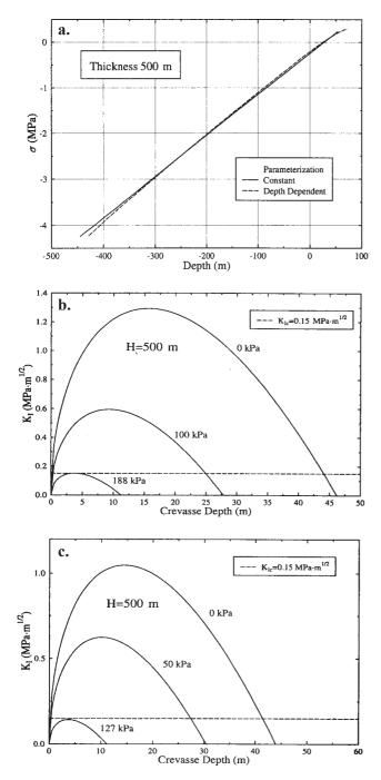
Fig. 9. a. Comparison of the stresses in floating ice of thickness 500 m depth dependent and constant ice density. Stress intensity factors are shown with the critical back stress necessary to retard fracture for **b**. the constant density case, and **c**. the depth dependent density case.
