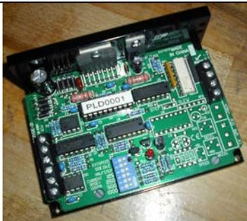
**Figure 12: Motor controller**
