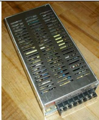
**Figure 13: Step motor power supply**
