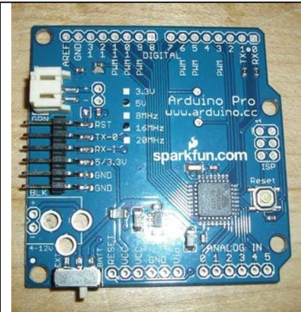
**Figure 14: Arduino micro controller**
