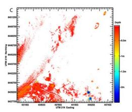
**Figure 1.** Meltwater depths derived using equation (2) overlaid on ASTER images acquired on (a) 29 June 2003 (b) 06 July 2003, and (c) 08 July 2004.
