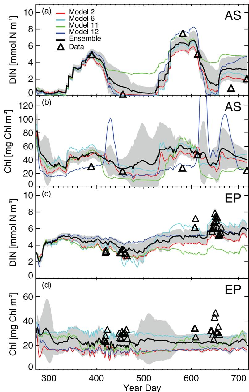
**Figure 4.** Simulations of (a,c) surface DIN and (b,d) integrated chlorophyll in the Arabian Sea (Figures 4a and 4b) and equatorial Pacific (Figures 4c and 4d) for models 2, 6, 11, and 12 plotted as a function of Year Day 1994 (AS) and Year Day 1991 (EP). Data (triangles) and the Ensemble Model time-series (mean of all 12 simulations) are shown for reference. Shaded area represents the Ensemble Model  $\pm$  one standard deviation.
